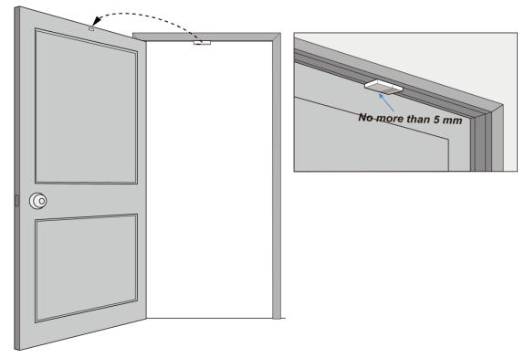
Avoid mounting WADC-1 on a metallic surface. If you choose to mount the device on a metallic surface, make sure to
