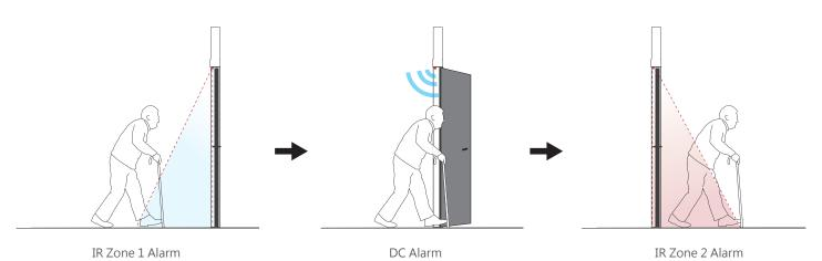
WADC-1 is a door contact that combines PIR sensors to monitor openings of the door and detect the movements around it. As an enhancement to comprehensive care for the elderly, WADC-1 is specially designed for those who are suffering from dementia and prone to wander, protecting them from potential risks.
